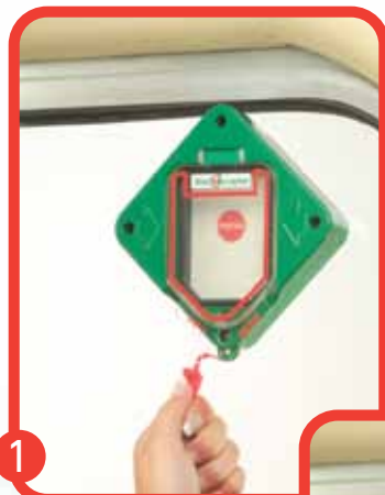
1 In an emergency, break security seal
